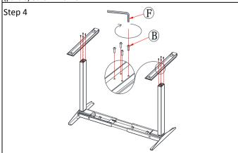
Attach Foot (part 1) to the Lifting leg (part 2) using (part B) Screw M6x16.
