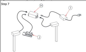
Connect the Lifting legs (part 2), Handset (part J), and the Power cable (part I) to the Control box (part H).
