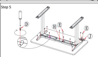
Adjust Crossbeams to the proper position to fit the desktop. Tighten the (part D) Wood screw ST4.8x19 to lock. Attach the Handset (part J) and Control box (part H) to the underside of the desktop using (part E) Wood screw ST4.2x16.
