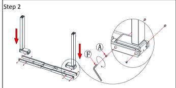
Attach the Lifting leg (part 2) to the Crossbeam (part 4) using (part A) Screw M6x10.
