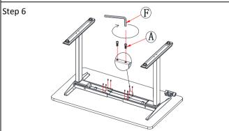
Tighten Crossbeams (part 4) using (part A) Screw M6x10.
