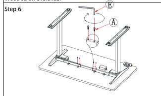
Tighten Crossbeams (part 4) using (part A) Screw M6x10.
