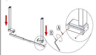
Attach the Lifting leg (part 2) to the Crossbeam (part 4) using (part A) Screw M6x10.
