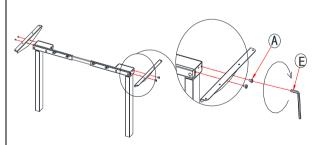
Attach the Side bracket (part 3) to the Crossbeam (part 4) using (part A) Screw M6x10.
