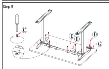
Adjust Crossbeams to the proper position to fit the desktop. Tighten the (part C) Wood screw ST4.8x19 to lock. Attach the Handset (part G) and Control box (part H) to the underside of the desktop using (part D) Wood screw ST3.5x12.
